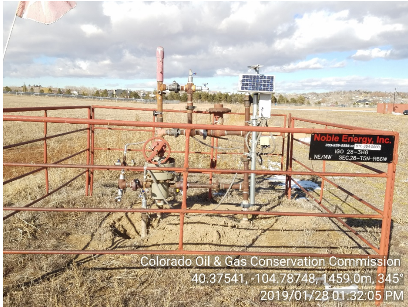
Photo #1 Igo 28-3H6 (05-123-18373) wellsite Shut-In | LOTO Weeds appear to be mitigated No Orange SI / TA tag per agreement
