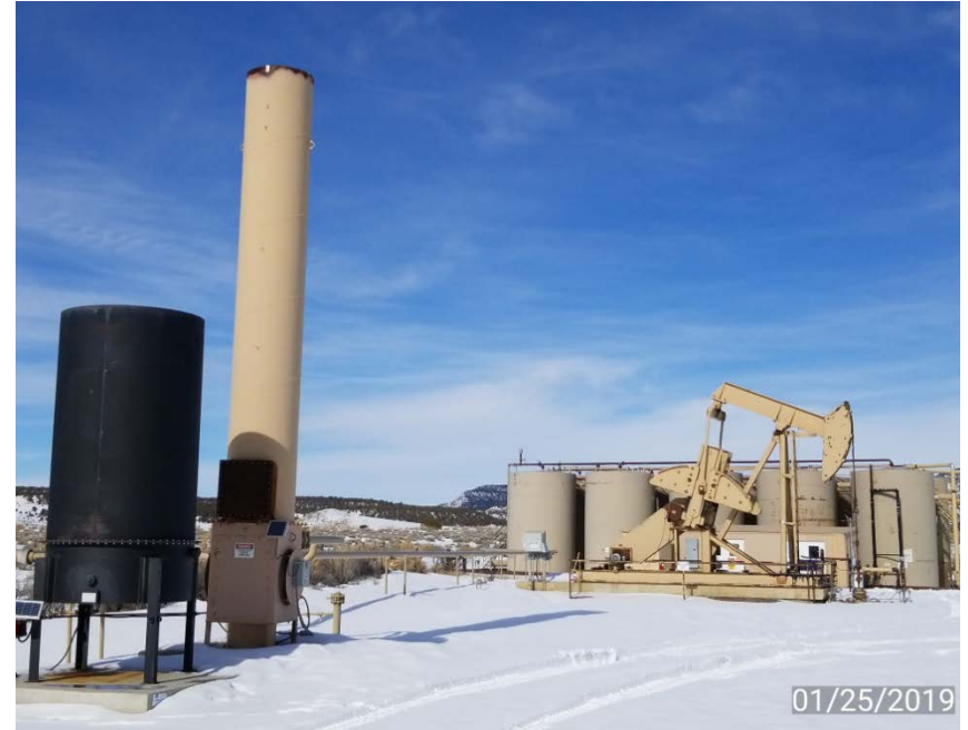
Photo 4. Emission control devices, pump jack, and injection well battery.
