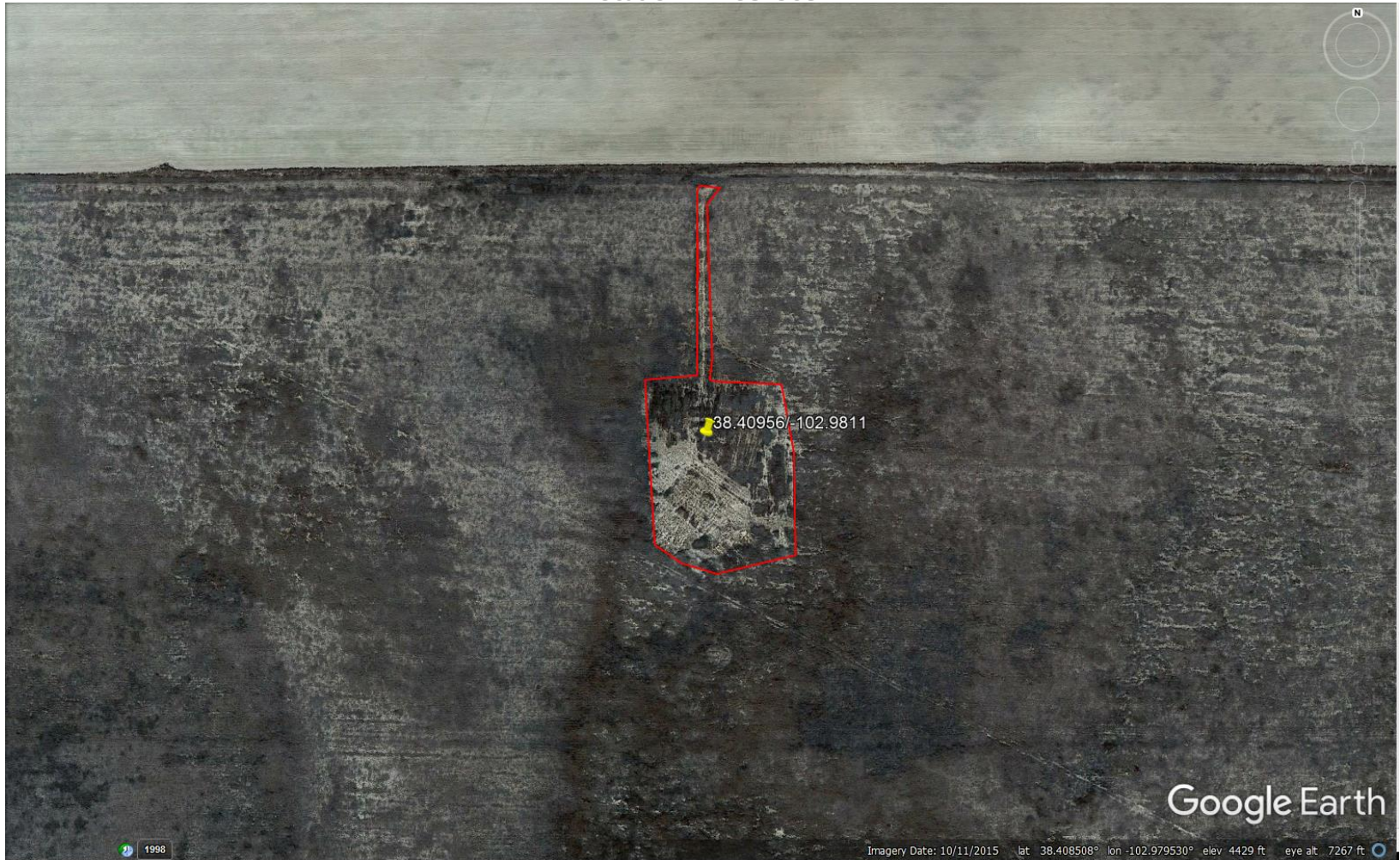
Photo 1: 2017 Google Earth aerial image. Photo shows areas of the location (red polygon, ~4 acres) where vegetation has not achieved a uniform desirable perennial vegetative cover. Photo also shows access road. Access road remains predominantly bare and exposed soil.
