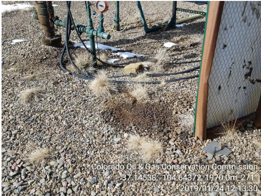
PHOTO 3: STAINED SOIL BETWEEN SOUND WALL AND WELLHEAD.
