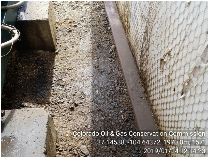
PHOTO 5: STAINED SOIL NEAR ENGINE SKID ON WEST SIDE INSIDE SOUND WALL.
