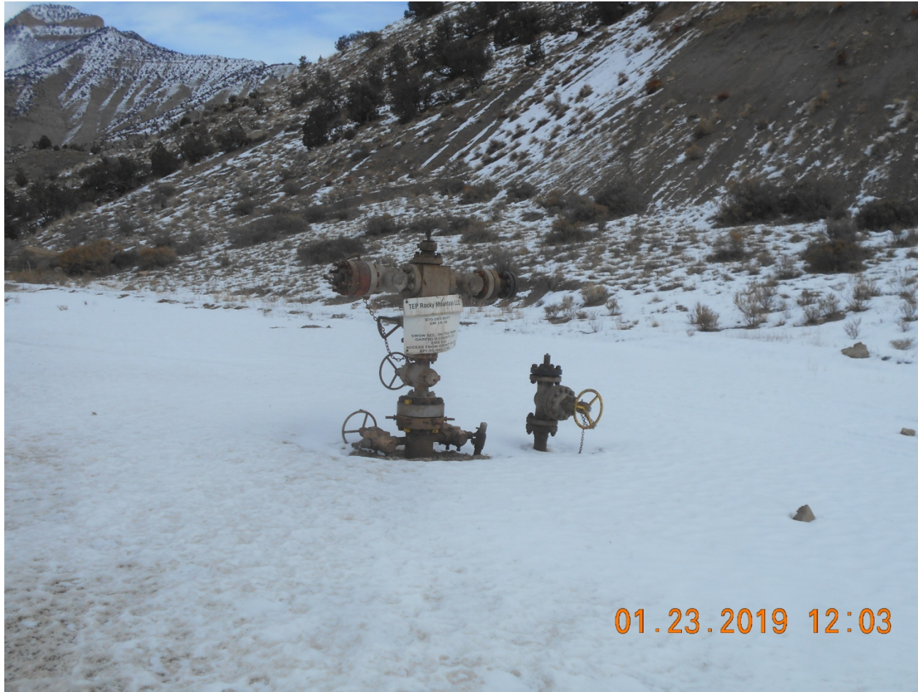
Injection wellhead
