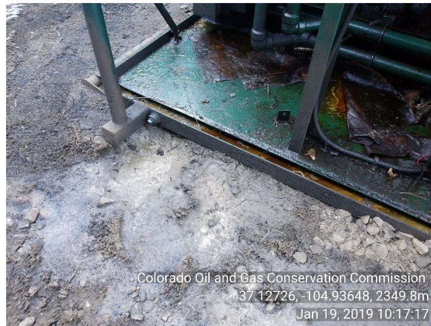
Photo 6 stained soil around liquid ring moto skid
