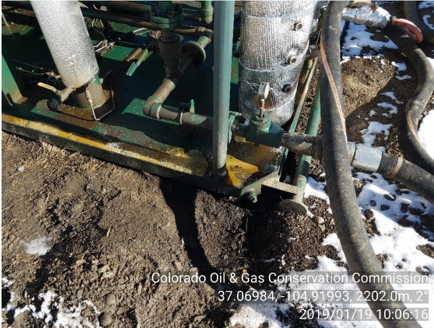
PHOTO 3: APPEARS TO BE STAINED SOIL IN HOLE NEAR DRAIN PLUG ON COMPRESSOR SKID
