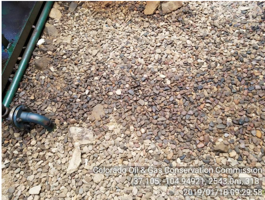
PHOTO 5: ANOTHER PHOTO OF STAINED SOIL NEAR COMPRESSOR SCRUBBER DRAIN
