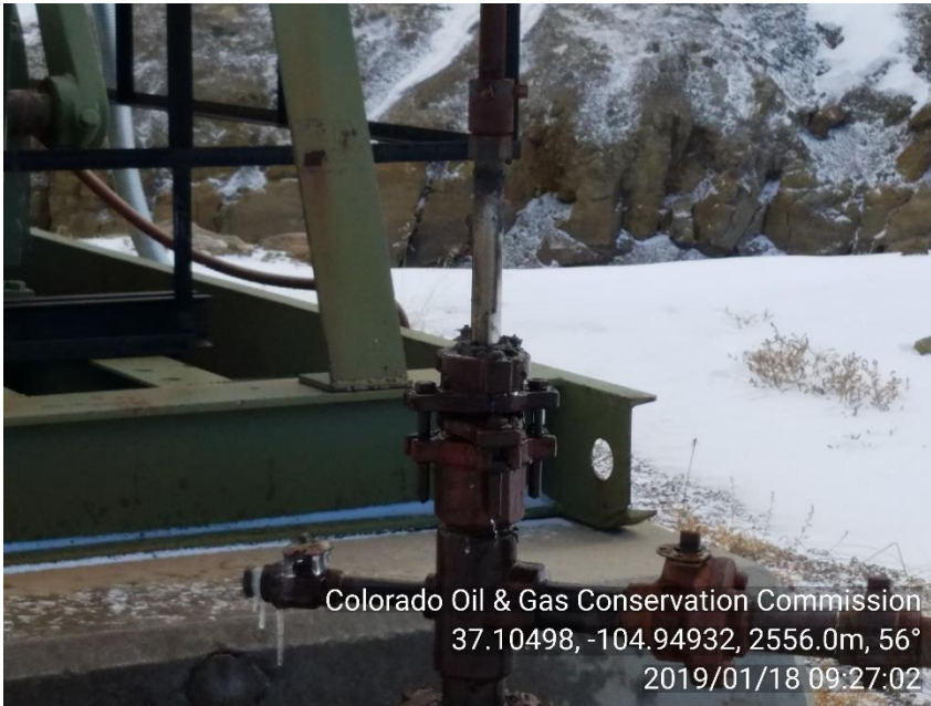
PHOTO 3: TBG HEAD PACKING LEAKING FLUID ONTO LOCATION
