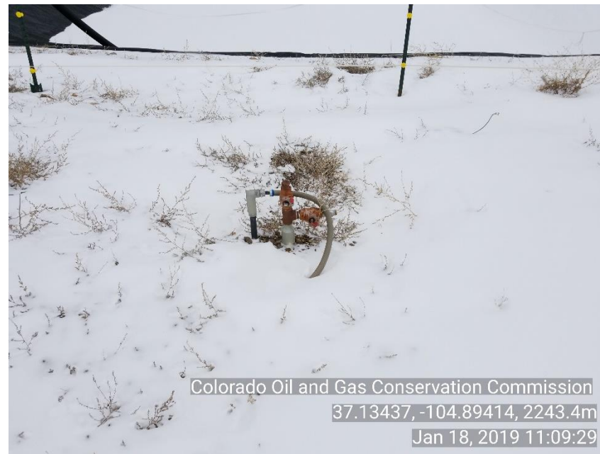
Photo 10 Unused, unmarked and not LOTO riser
