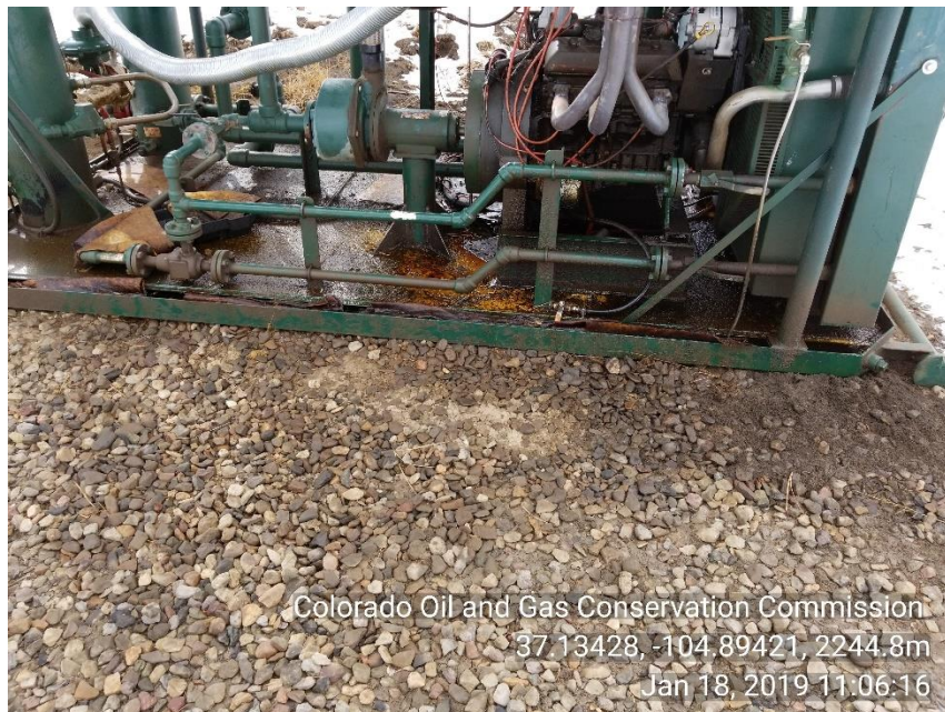
Photo 3 Stained soil around liquid ring
