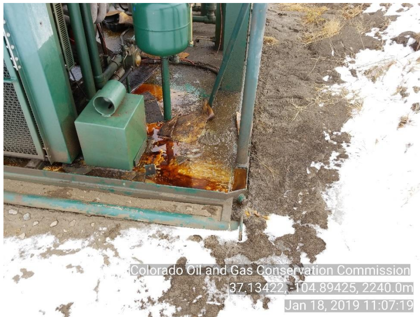
Photo 5 Stained soil around liquid ring and fluid dripping out of skid
