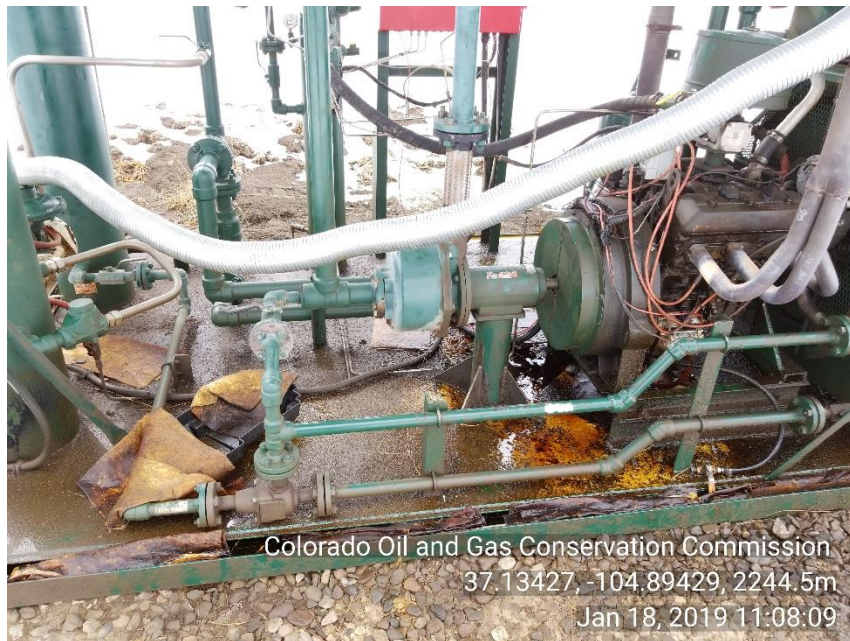
Photo 7 trash and debris inside liquid ring skid
