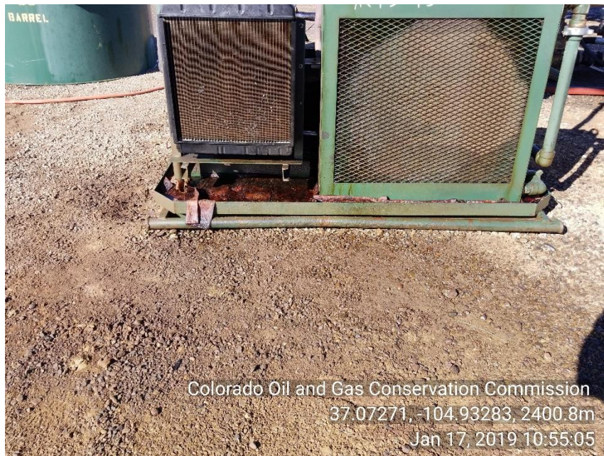
Photo 9 stained soil in front of liquid ring compressor
