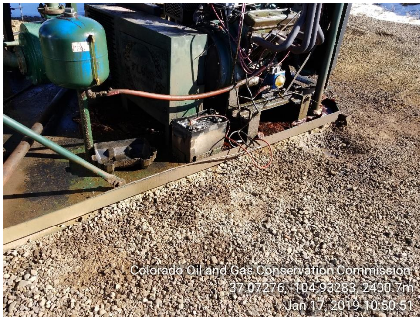
Photo 5 Stained soil around liquid ring compressor
