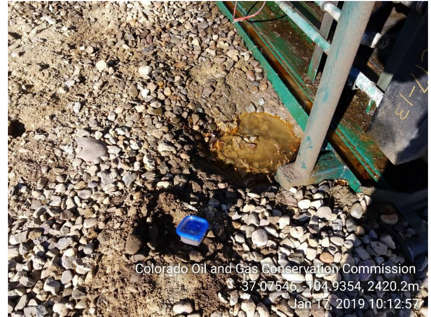
Photo 6 soil sample taken by drain plug to liquid ring
