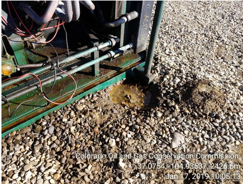
Photo 5 Stained soil around drain plug of liquid ring
