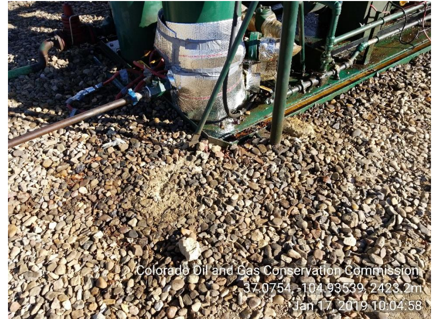
Photo 4 Stained soil around liquid ring
