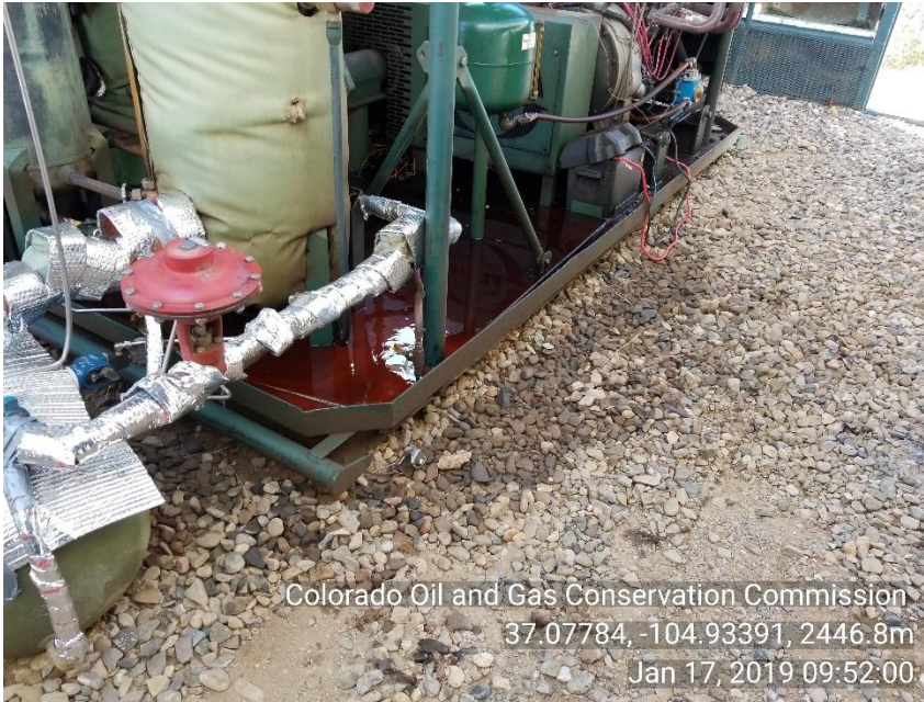
Photo 5 Stained soil around liquid ring compressor
