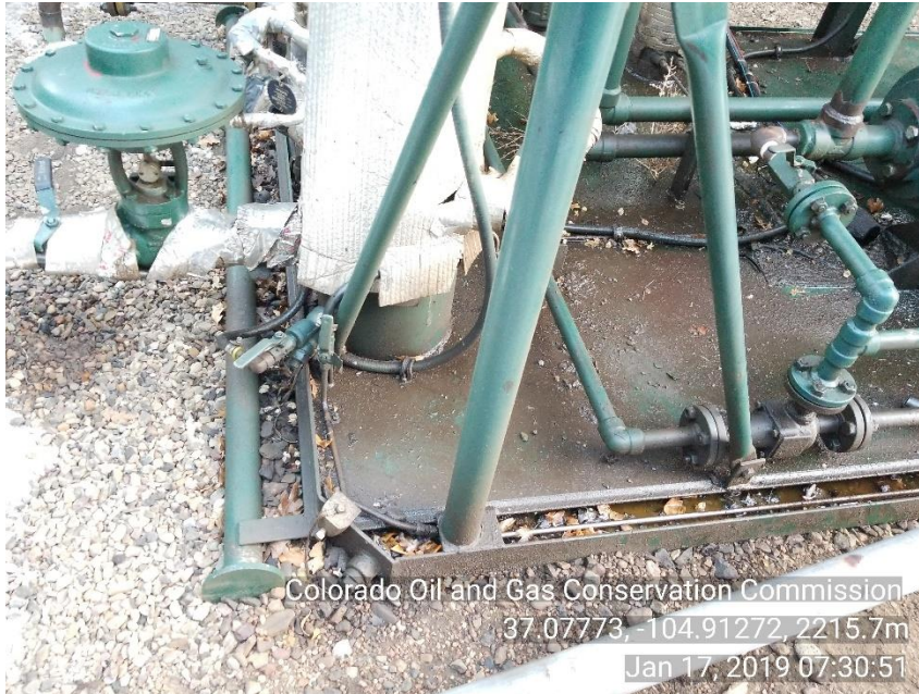
Photo 3 Stained soil around skid
