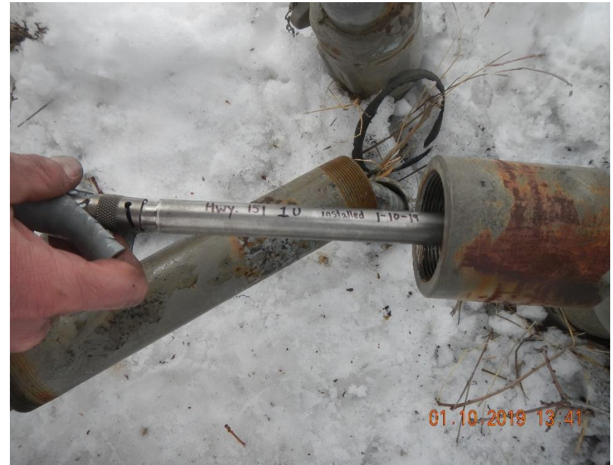
New Level Troll 700 series 1000 psia pressure transducer installed in upper position in monitoring well #1.
