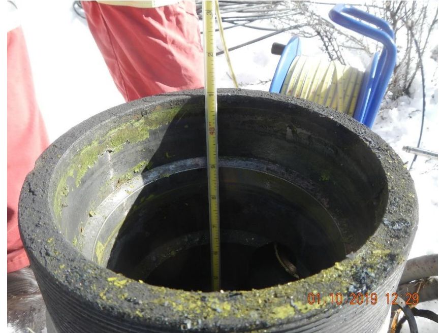
Water level measured at 43.10' from top of casing with 1.45' stick up from top of collar.
