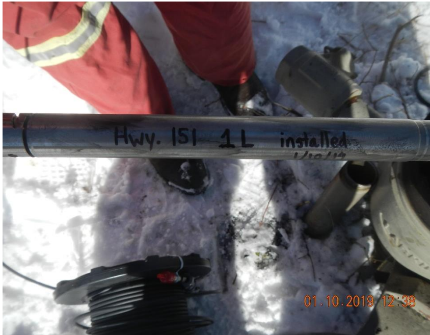
New Level Troll 700 series 1000 psia pressure transducer installed with 285' new rugged cable in monitoring well #1.
