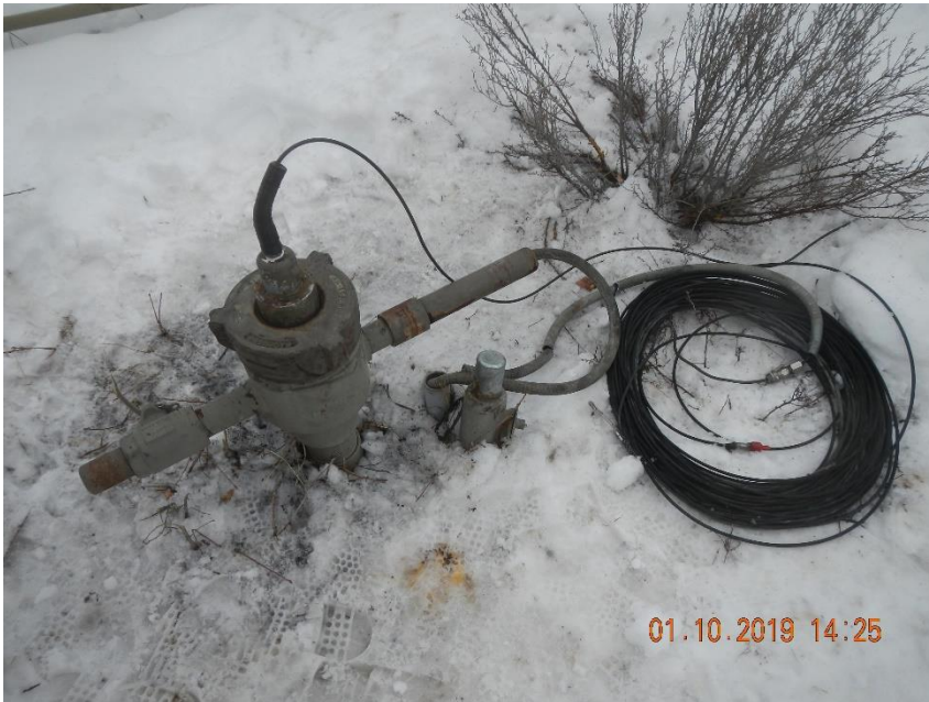
Monitoring well #1 after equipment replacements.
