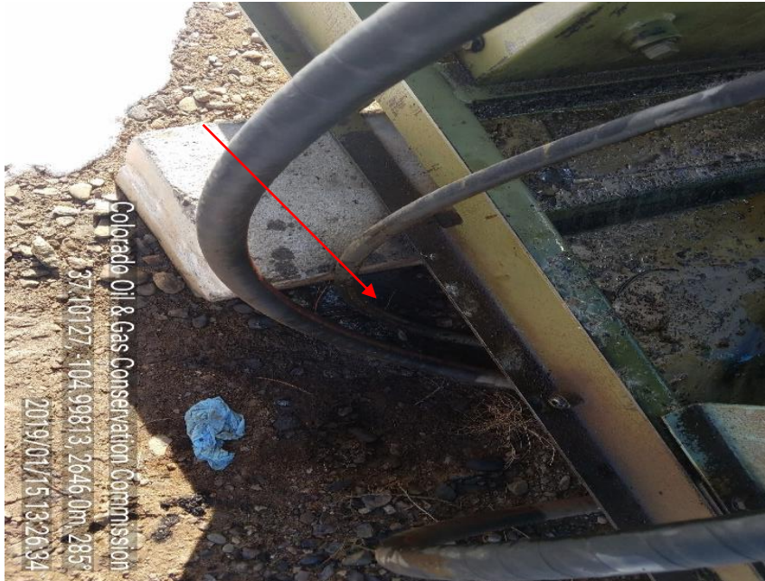
PHOTO 3: STAINED SOIL NORTH SIDE OF ENGINE SKID
