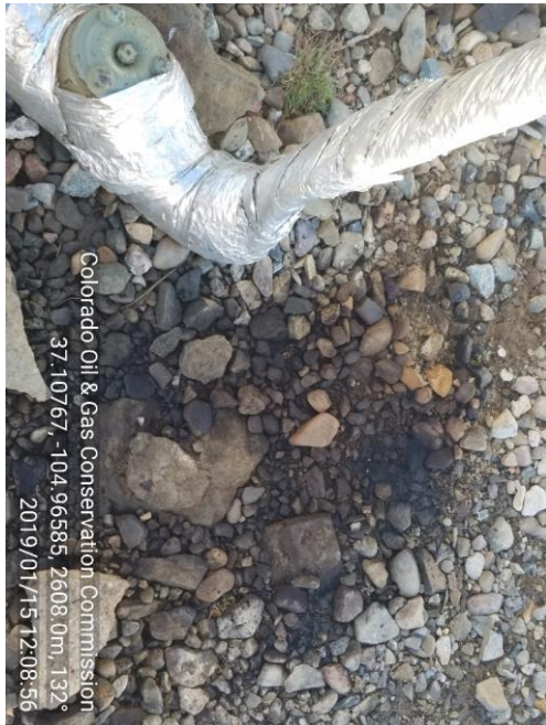
PHOTO 3: STAINED SOIL WEST SIDE OF COMPRESSOR SKID IN FRONT OF SCRUBBER
