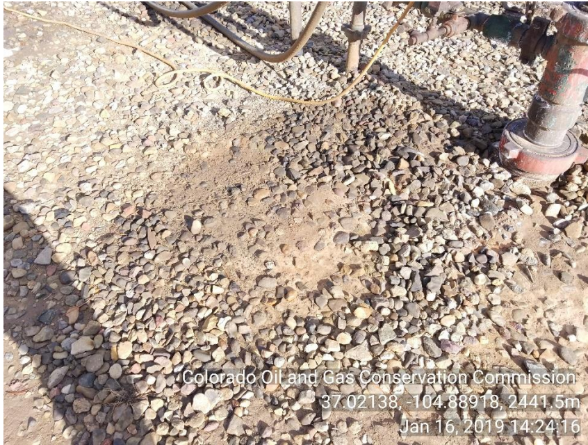
Photo 3 stained soil under HYD fittings on WH
