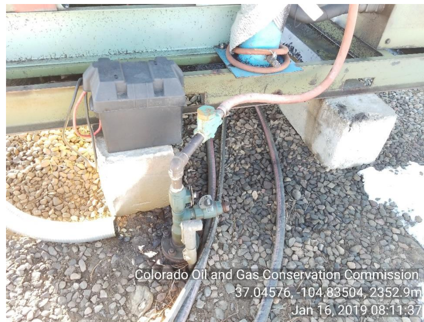
Photo 4 Stained soil under drip pot
