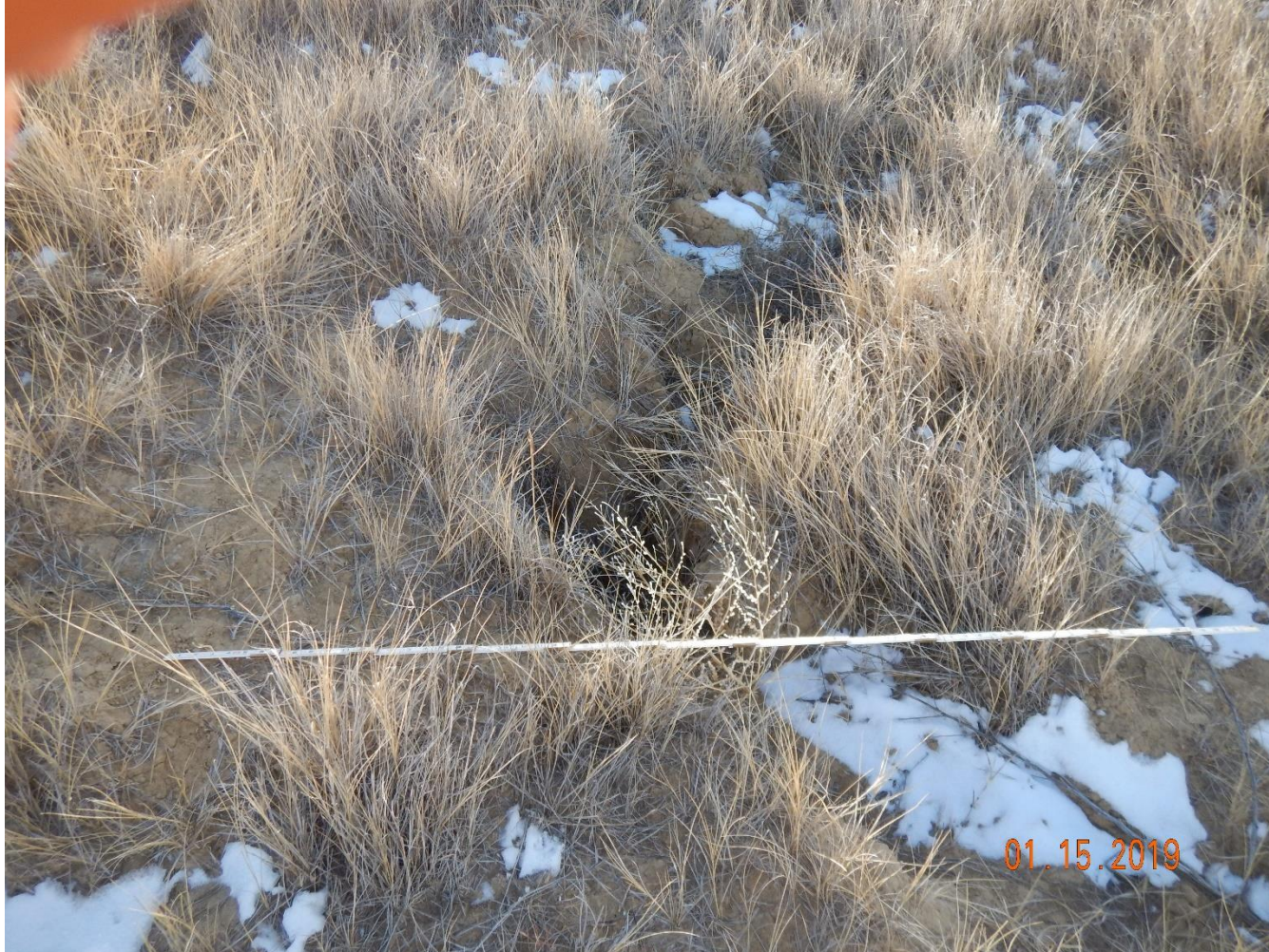
Photo 4: Photo taken from the cut slopes on the southeast corner of the location. Corrective actions required operator to repair erosion degradation and conduct revegetation activities on the cut slopes of the location. Photo shows stormwater erosion has not been repaired/stabilized, and BMPs have not been installed/maintained. Stormwater has been allowed to continue, and has continued to degrade the location. Photo also shows additional revegetation activities to stabilize slope has not been conducted. 6 foot measuring stick for reference.
