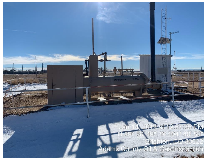
Photo#2 Separator/Gas Meter/Automation RTU
