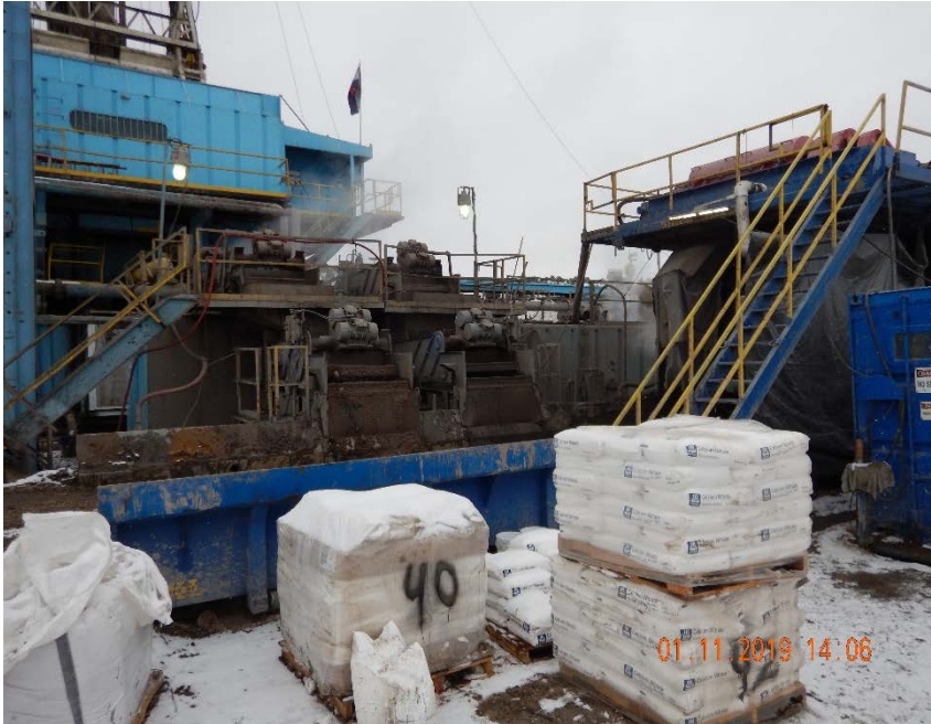
Photo #5 – View of drilling rig and cuttings shaker from south.
