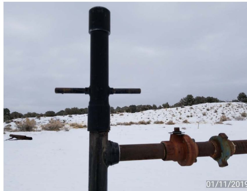
Photo 2. Gas leaking along bottom threads of plunger.
