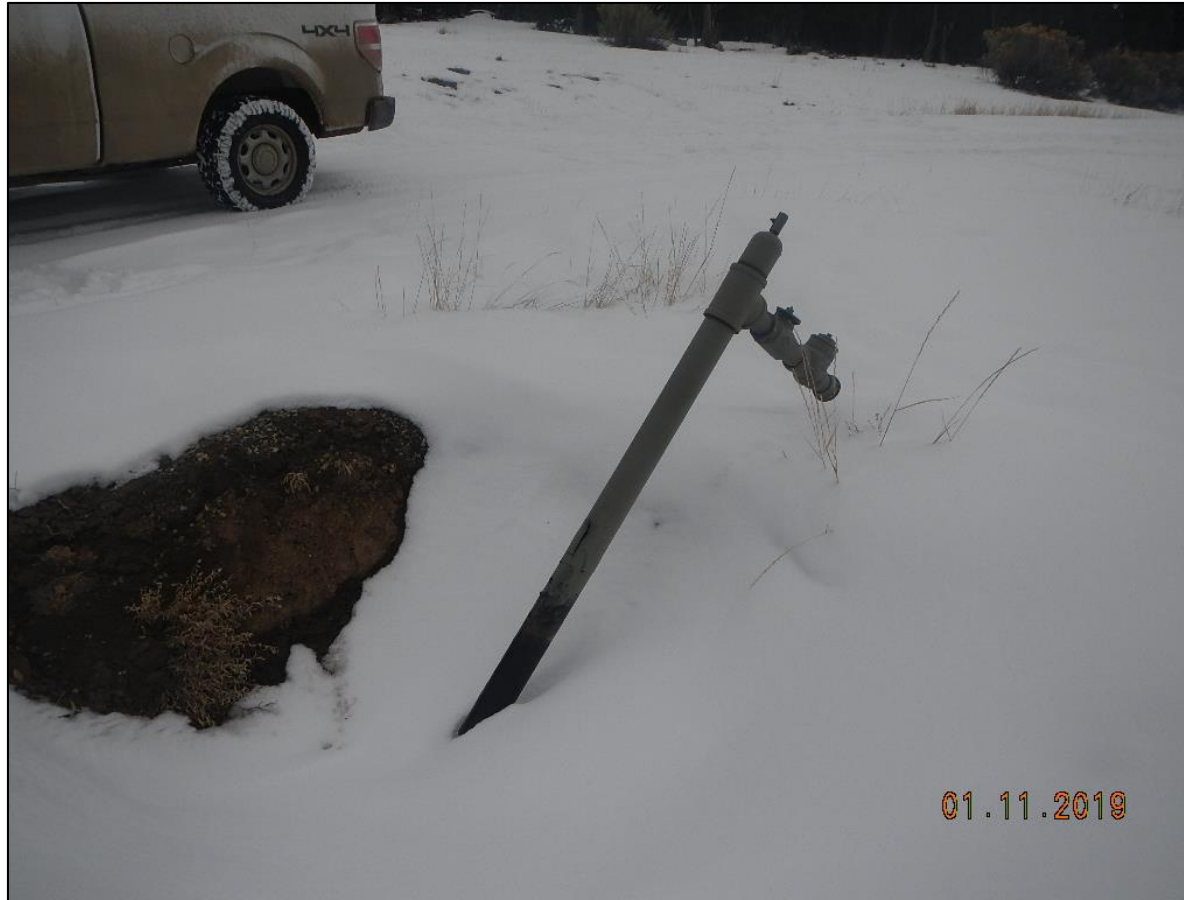
Unmarked riser left on location with hole in ground
