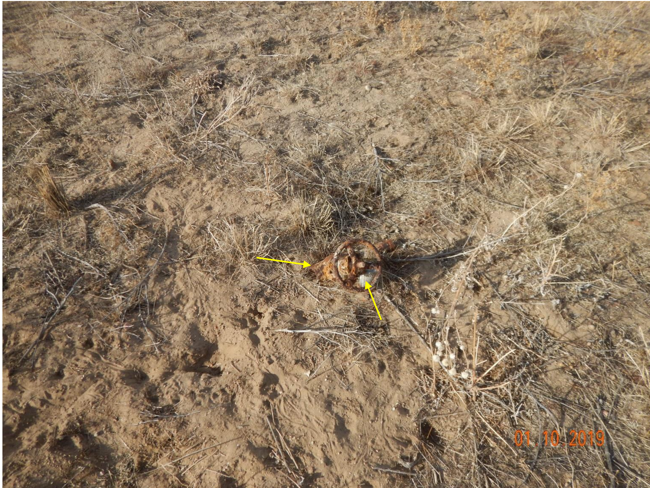
Photo 5: Photo taken from the well location. Photo shows a valve (debris) and a riser that have been documented and required removal in previous inspections. Photo shows valve and riser have not been removed.
