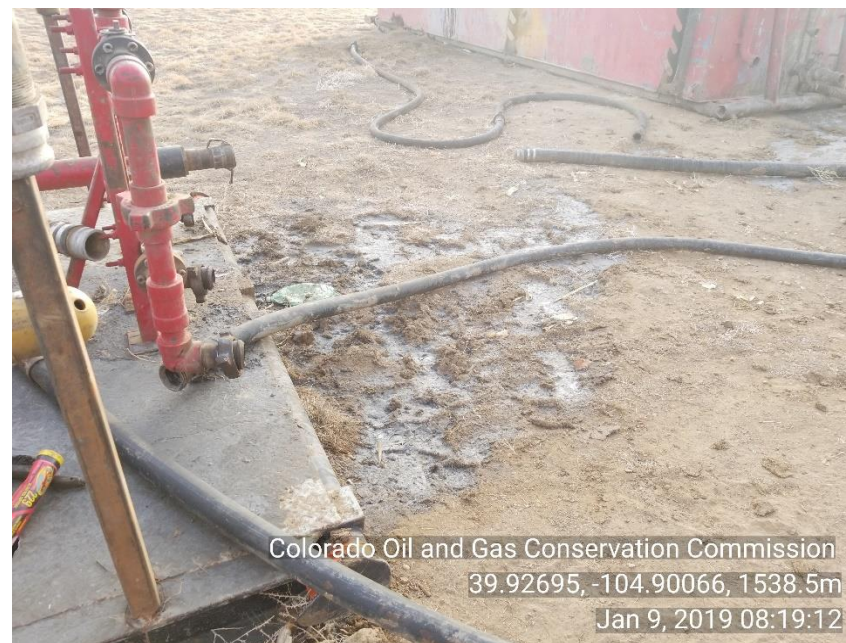
Photo 4 Fluid around Pump
