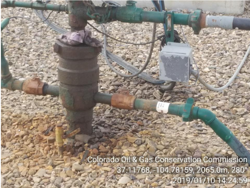
PHOTO 3: STAINED SOIL AROUND WELLHEAD
