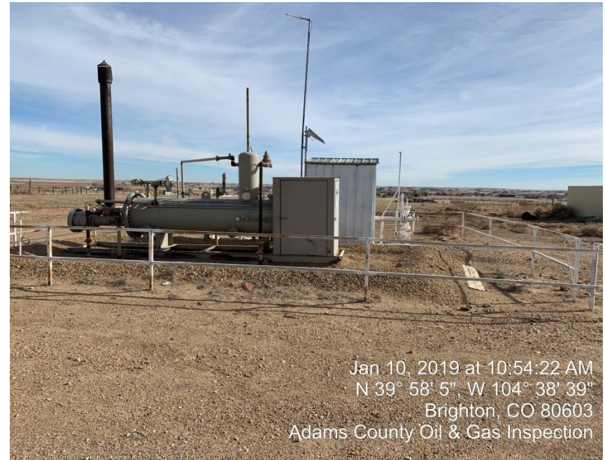
Photo#2 Separator/Gas Meter
