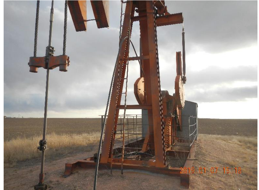
Photo 8: Above ground supply gas line ran through pumping unit.
