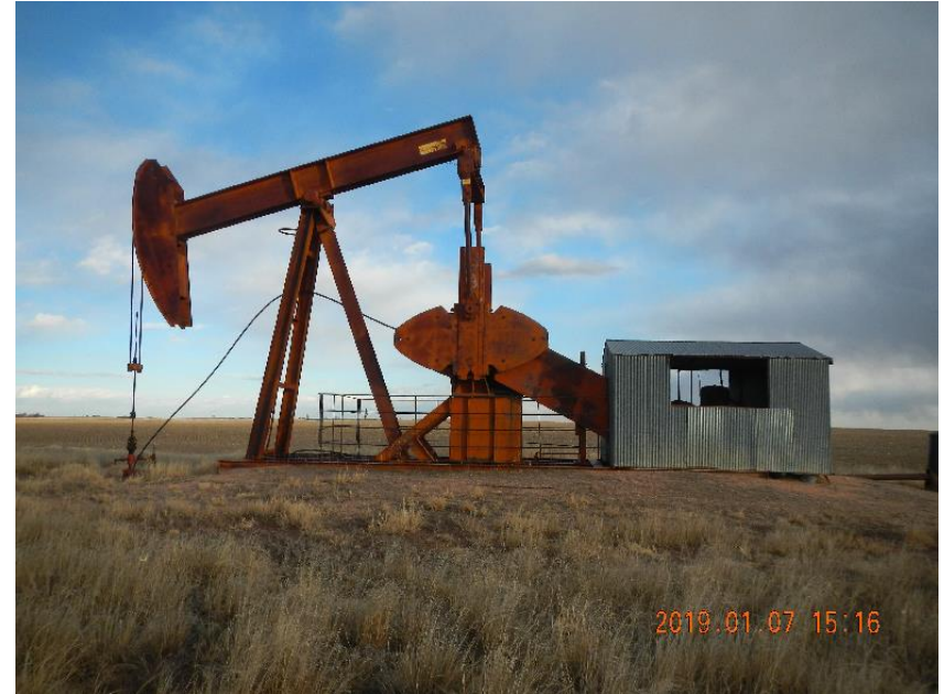
Photo 4: Pump jack and metal prime mover shed and above ground supply gas flowline visible from wellhead and running through pumping unit.
