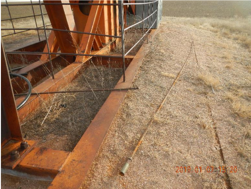
Photo 9: Rod section off R side of pump jack.
