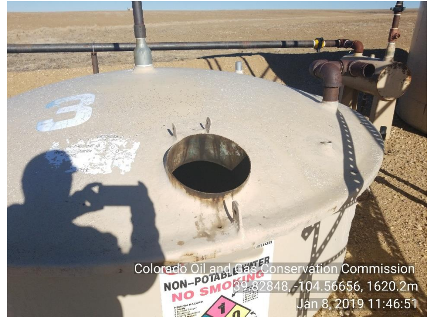
Photo 4 Gauge Hatch missing H2O tank
