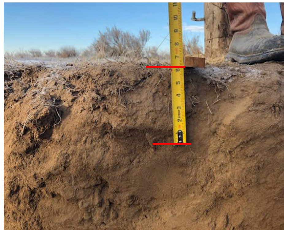
Photo NBL2 - Topsoil depth at west edge of pad, estimated at approximately 6 inches.
