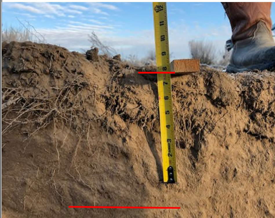
Photo NBL1 – Topsoil depth at south edge of pad, estimated at approximately 10 inches.
