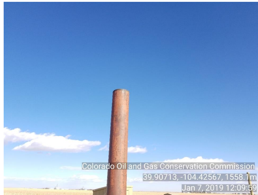
Photo 6 not bird netting on sep stack
