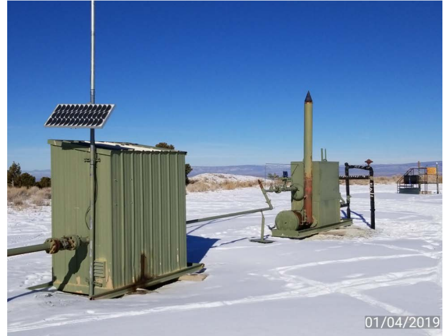
Photo 2. Gas meter, separator, well head.
