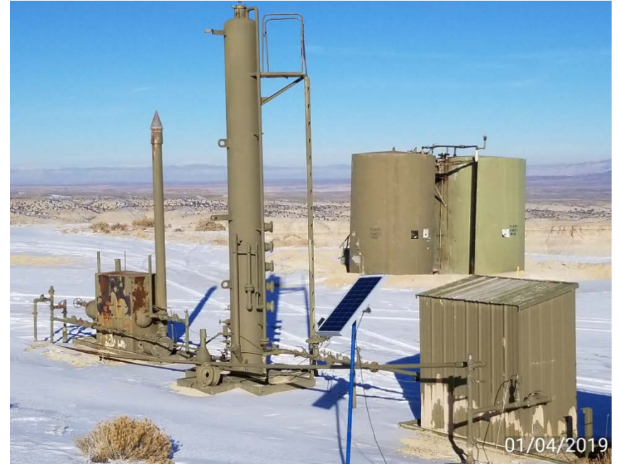
Photo 4. Separator, gas meter building, tank battery.
