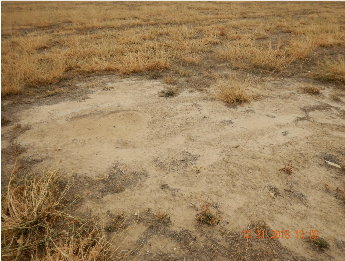
Photo 1. Photo taken from the well location, facing West. No equipment observed at the well location. Photo illustrates subsidence at the PA well location with no vegetative growth.
