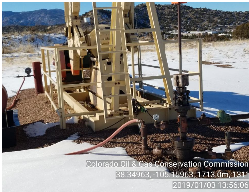
PHOTO 1: WELLHEAD/ STAINED SOIL AT WELLHEAD
