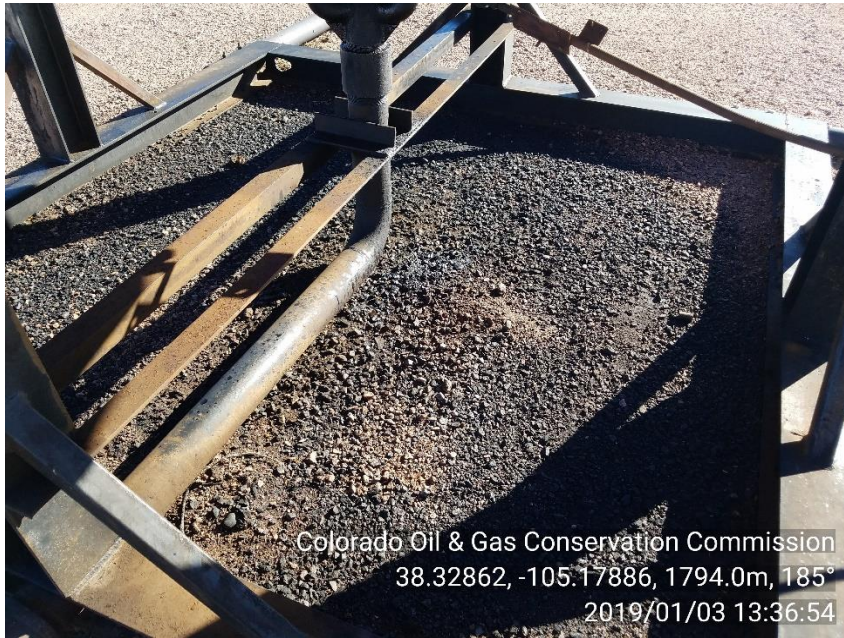
PHOTO 3: STAINED SOIL UNDER ECD
