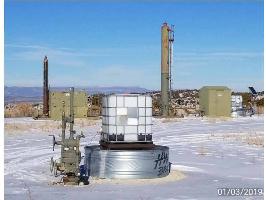
Photo 2. Well head, separator, and gas meter building.
