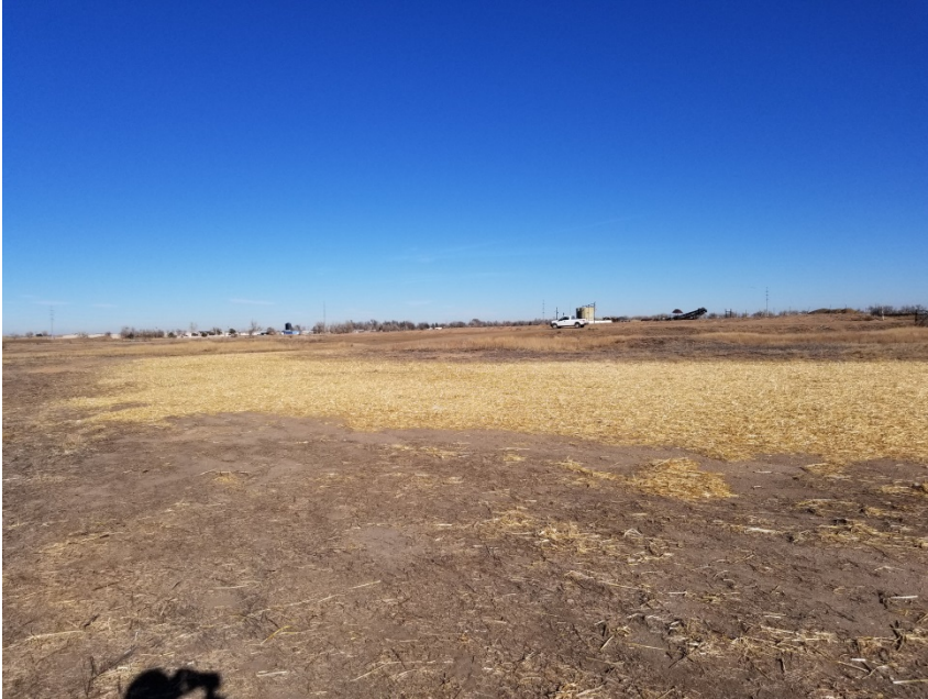
Photo 1. Photo taken from the location, facing North. Appears the Operator has performed final reclamation activities, with the evidence of drilling rows and straw crimped mulch. However, approximately half of the location and access road have no indication that compaction alleviation or reclamation was performed.
