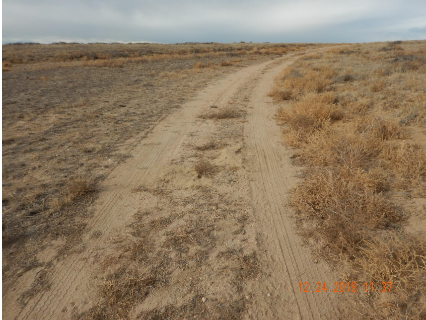
Photo 1. Photo taken from the main access road (shown in the aerial image), facing West. Operator has failed to reclaim the access road per Rule 1004 standards (e.g., recontour, decompact, etc.). Wind erosion was observed along portions of the main access road.
