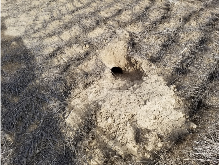
Photo 3. Photo taken from the location showing the test pit dug to check on decompaction. See comments from Photo 1.
