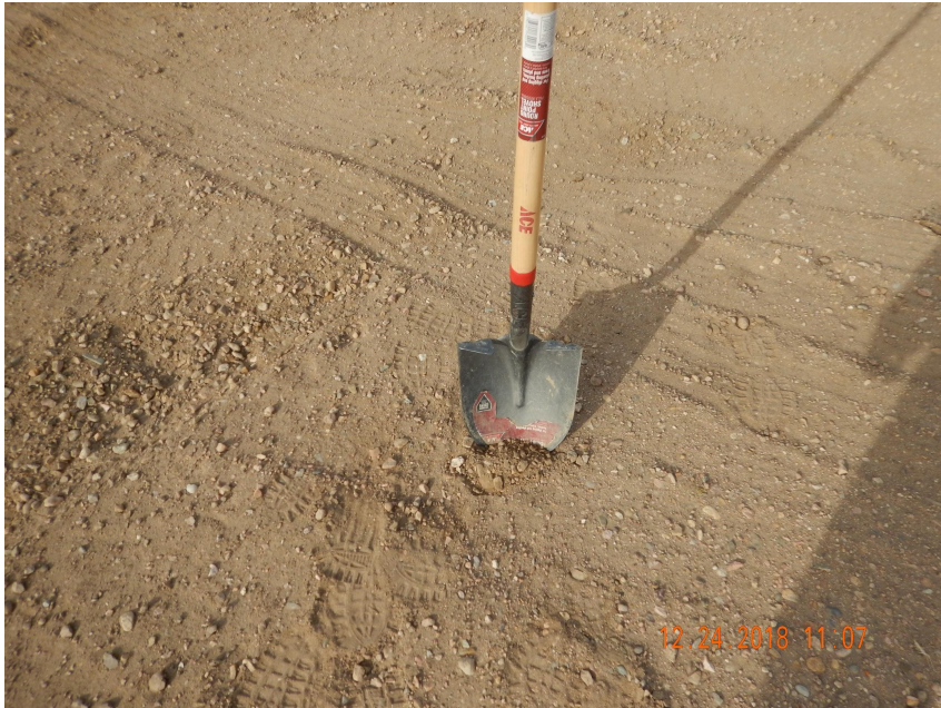
Photo 2. Photo taken from the former plugged and abandoned location. Photo illustrates gravel has not been removed and decompaction has not been performed. COGCC Staff could not penetrate the shovel more than a couple inches into the surface.
