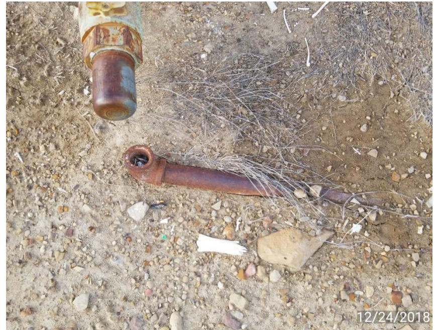
Photo 2. Riser next to well head not capped or LOTO.
