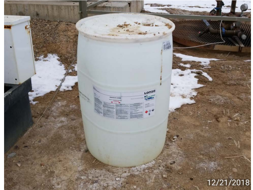
Photo 2. Barrel stored on location without secondary containment.
