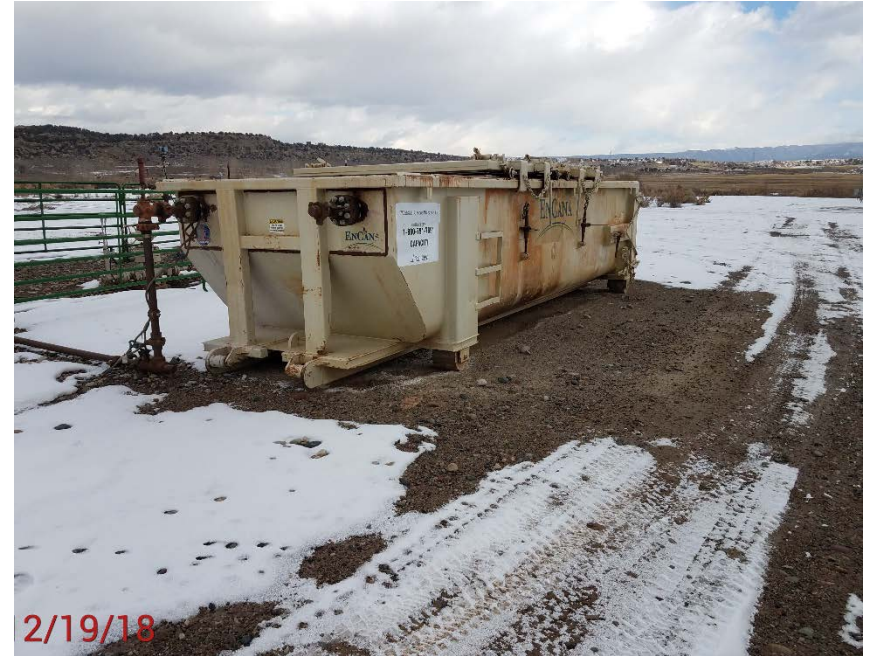
Location Photo #4, No secondary berm around tank
