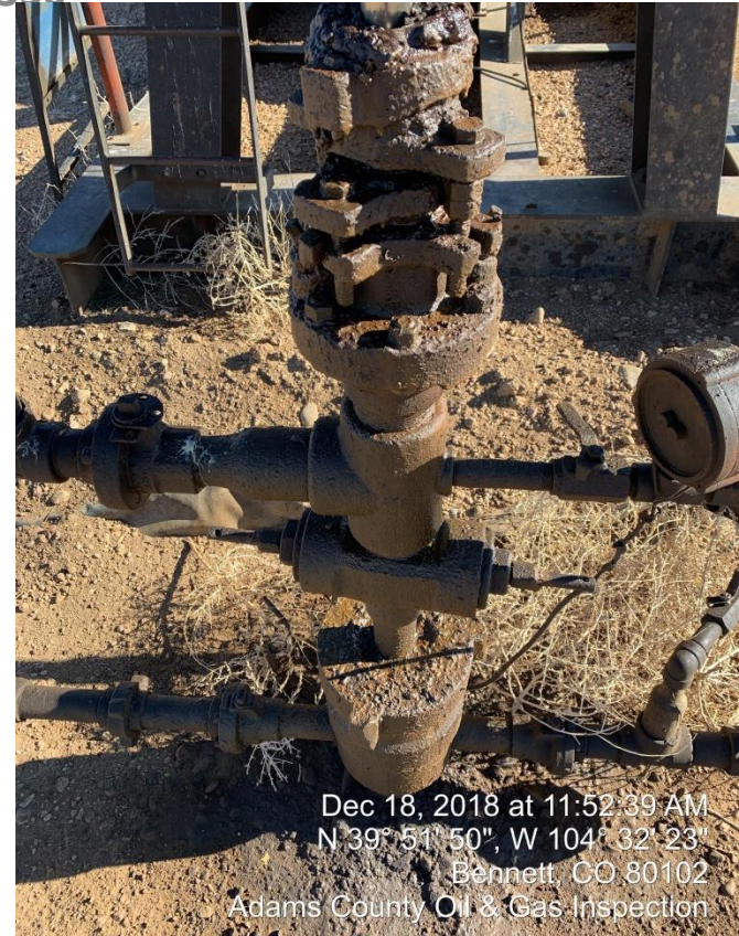
Photo#2 Corrective Action: Wellhead leaking/Stained Soil
