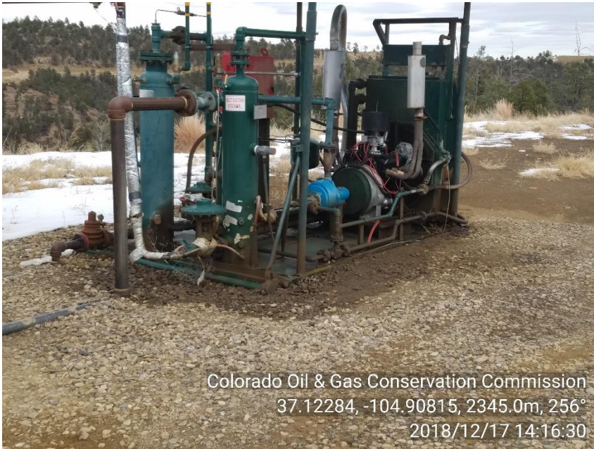
PHOTO 3: STAINED SOIL AROUND COMPRESSOR
