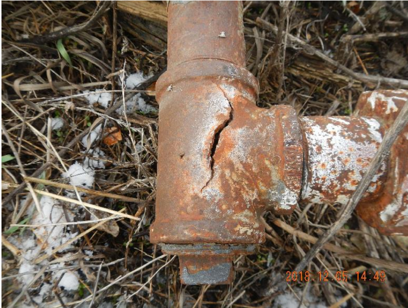
Photo 3: Close up of damaged T.
