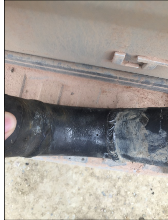
90 Degree elbow where pin hole was found. Pin hole was on inside radius of elbow
