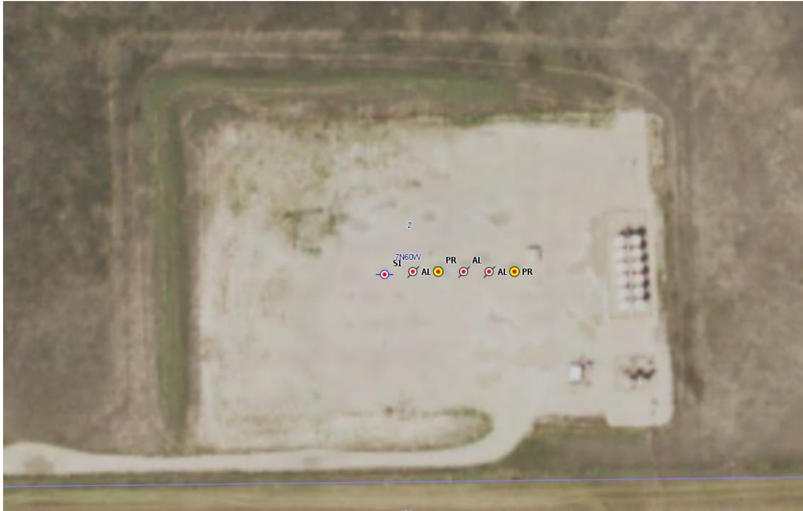
Photo 8: 2017 COGIS aerial imagery. Photo shows areas on the west end of the location that do not appear to be necessary for production operations. These areas need to be reclaimed in accordance with COGCC 1003 interim reclamation requirements.
