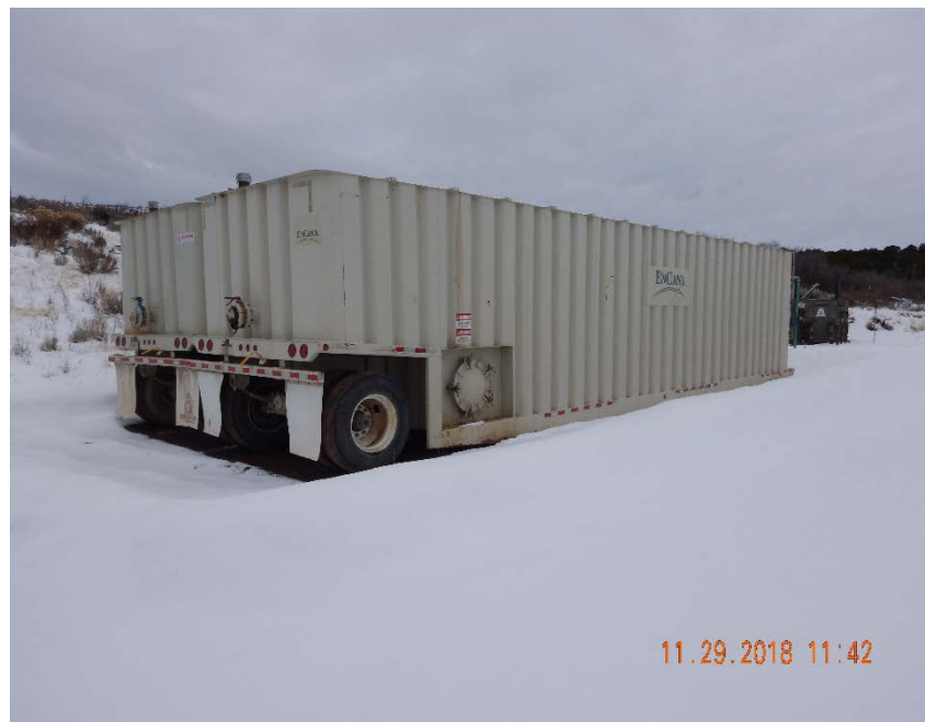
Photo #5 – Temporary tanks are being used on pad until tank battery can be rebuilt after remediation is complete.
